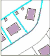
Tracing features in ArcMap. No offset is used in this example.
