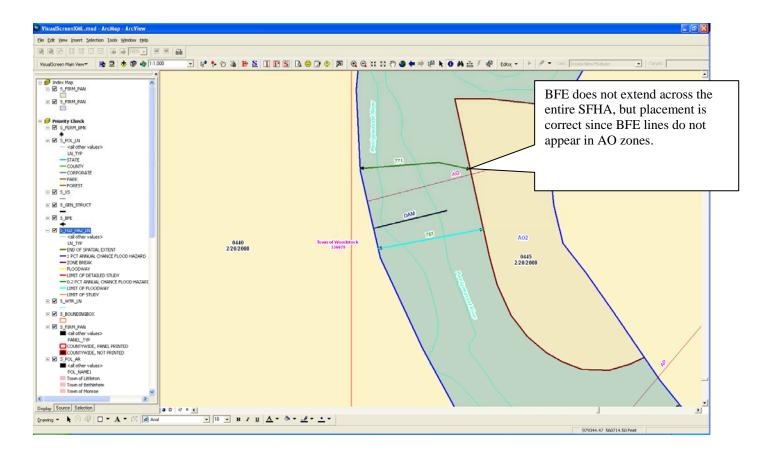
Another example of where the BFE line does not extend across the entire SFHA, but the placement is actually correct is presented below. In this case, BFE lines end at a levee. Since the BFE value is different on either side of the levee, these lines will be allowed to pass as long as the end points are within 25 feet of a S\_GEN\_STRUCT feature:
