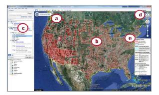
Figure 1. Opening view for the FEMA NFHL utility. Areas of interest include the (a) Quick Start Guide, (b) status map overlay, (c) "National Flood Hazard Layer (FEMA)" folder, (d) navigation controls, (e) eye altitude readout, and (f) map legend.
