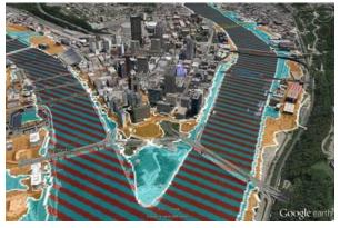
Figure 6. Three-dimensional view of flood hazard areas for Pittsburgh, Pennsylvania. Both flood hazard mapping and Google Earth use terrain data, but the data most likely are different. There may be discrepancies in views that display flood hazard and Google Earth data.
