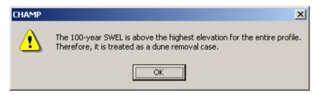
Click on OK to remove the dune and follow the instructions above for selecting the toe and drawing the eroded profile.
