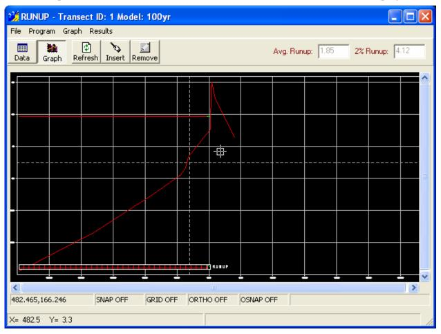
This plot shows the profile used in the runup analysis in red and the computed runup elevation (average computed runup depth plus SWEL) as a red dashed line. Click on the <u>Data</u> button to return to the RUNUP input window
